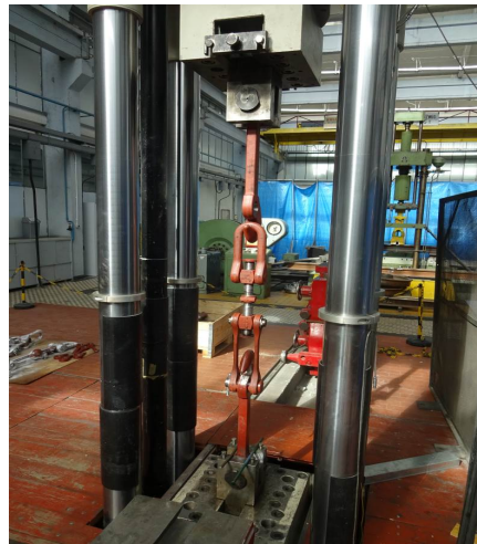
Fig. 1. Screw coupling 1MN on the testing machine during tests
