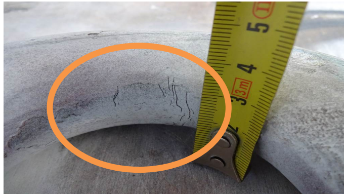
Fig. 3 Non-destructive testing NDT - magnetic-powder method, observations of the shackle screw coupling IMN after fatigue tests. Visible cracks in the marked area.
