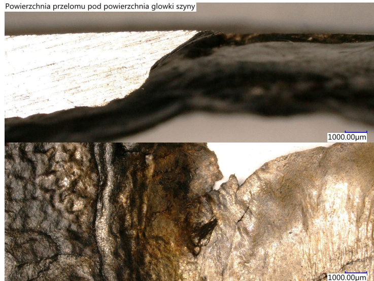
Fig. 3 Head checking defects occurring in the rail head - cross-section (top) - destruction zone under the surface of the rolling zone approx. 2 mm (microscopic observations) - (bottom).
