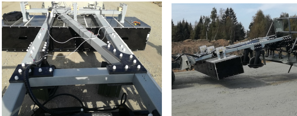
Fig. 3. Loaded frame with strain gauges (on the left) and the frame during tests (on the right)
