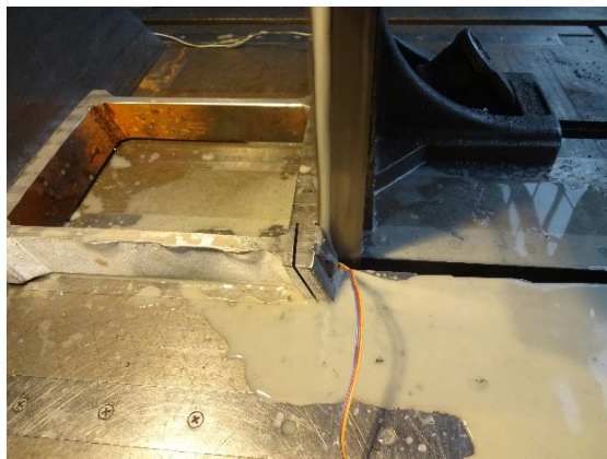
Fig. 1. Phase 4 – the last strain gauge cutting operation. Cutting the strain gauge out of the frame.
