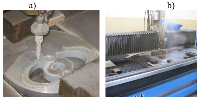
Fig. 4. Shaping of non-circular cogbelt pulleys: a) cutting a cogbelt pulley with a jet of water with an abrasant, b) CNC machine used for machining
