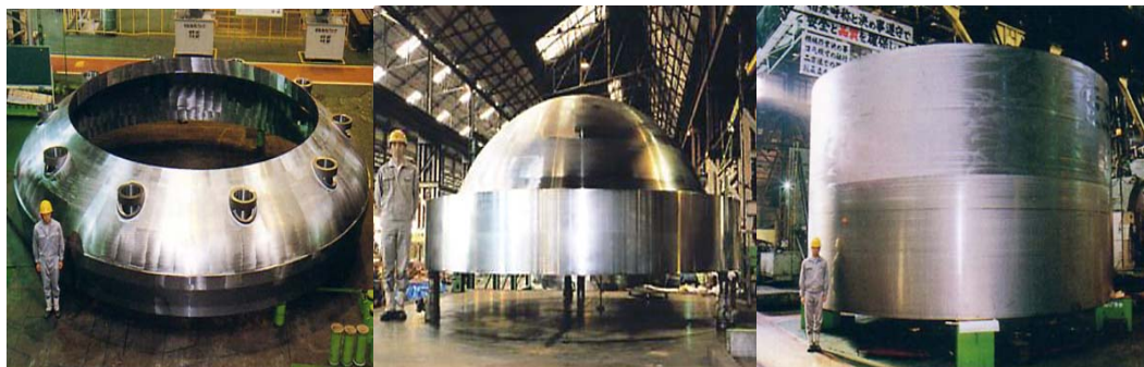
Fig. 6. Examples of forged parts for Reactor Pressure Vessels. (Left) Core region shell, (Center) Bottom petal, (Right) Closure head.
