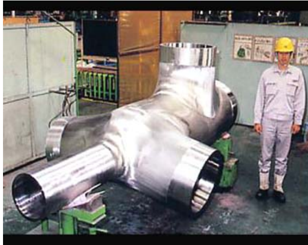
Fig. 7. PM/HIPP-NNS Offshore Deep-Sea Manifolds.
